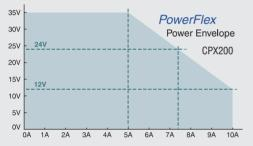
The CPX200 can provide up to 350 watts (175W per channel). As the set voltage is reduced below 35V, the maximum output current is increases up to a maximum of 10A.
